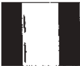
Appearance on the X-ray picture A thin dark line with sharp edges. Depending on the fault orientation in relation to the X-radiation, the line might give a blurred appearance.
