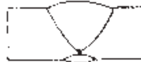
Root defects Incomplete penetration at the root or a gap which was not filled by weld metal.
