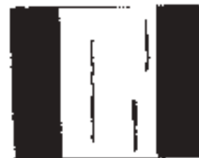
Appearance on the X-ray picture Long, more or less contours parallel with the weld.
